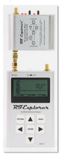
The RF Output of the Upconverter must be connected to the RF Input of the Analyzer.
