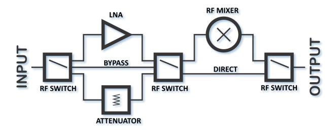
The internal RF blocks are connected by high performance RF switches. These are operated indirectly by push buttons to select the RF signal path.
