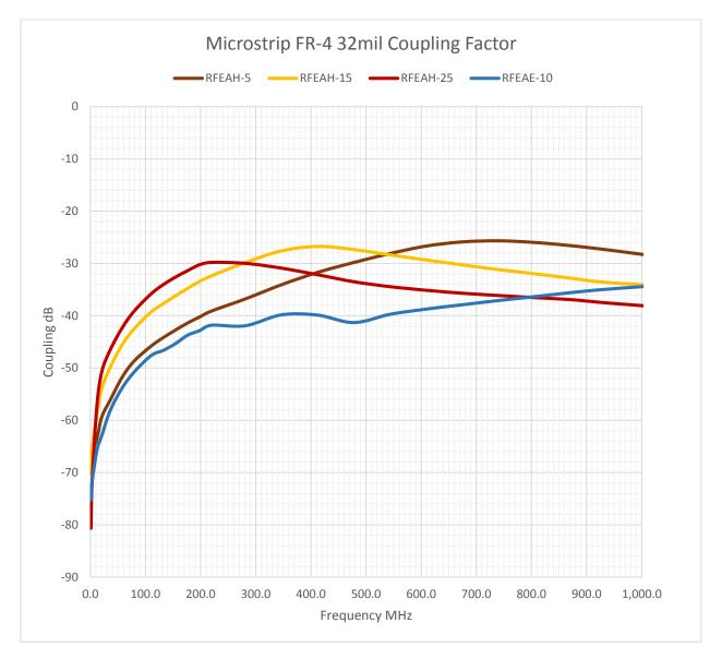
From the response graph above, covering 1GHz band – usually the most used for EMC and sniffing diagnosis:
