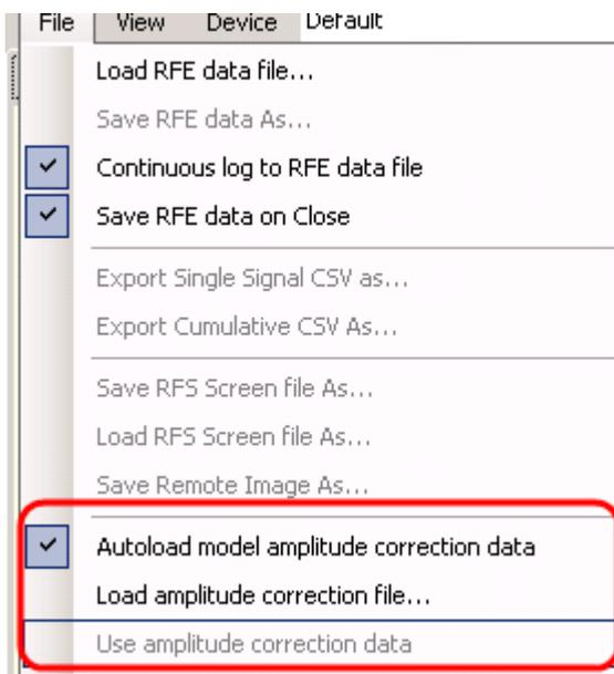
The RF Explorer for Windows automatically reads the right file and applies the correction to the measurement. For that to work, make sure to have the “Autoload model amplitude correction data” checked in the File menu and also check on “Use amplitude correction data” for the calibration files to effectively adjust all measurements.
